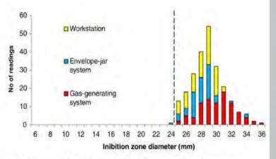
Reproducibility results from 18 laboratories and different anaerobic environments. Metronidazole 5 µg inhibition zone diameters on FAA-HB and Clostridium perfringens DSM 25589 (n=236)
